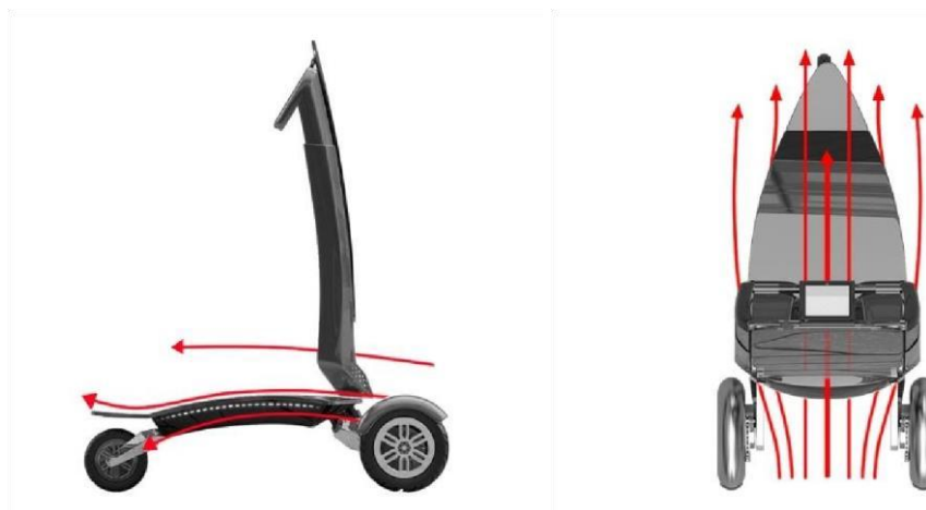
Fig. 37: Airflow relative to the scooter body construction
