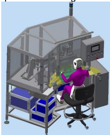
Fig. 4.21 System for assembly of a unit consisting of a seal, nut, and stud – front view
