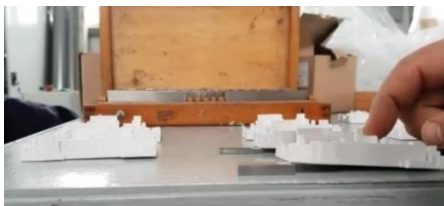
Fig. 2.6 Deviation from flatness of 5 mm compared to 0.4 mm specified in the drawing.
