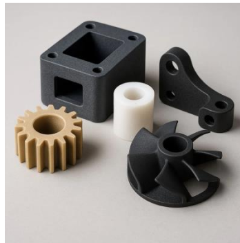
Fig. 2.19 Polymer parts produced by 3D printing
