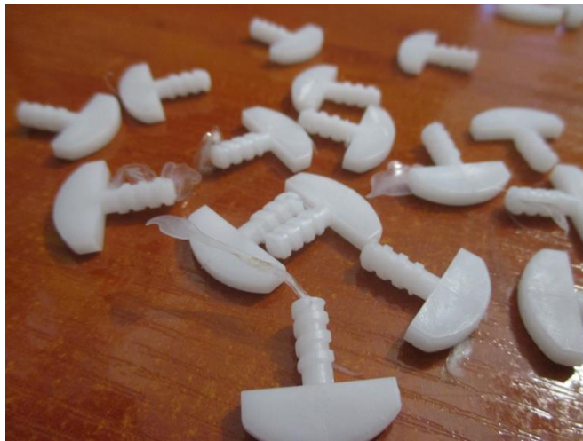
Fig. 2.5 Flash along the parting line
