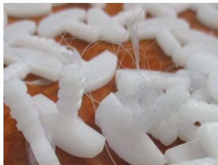
Fig. 2.8 Characteristic “stringing” occurring during the molding of POM material.
