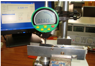
Fig. 7.3 Demonstration of the principle of operation of a proportional control head in Microtechnics and Micromechatronics classes.
