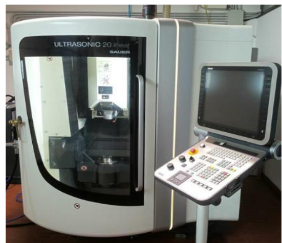
Figure 10-12: Multifunctional machining center for producing implants of hard and ultra-hard materials.
