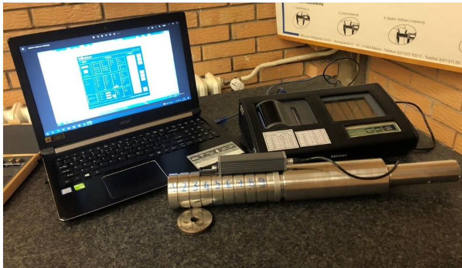
Figure 4. 3 Surface roughness measurements with Mitutoyo SJ-310
