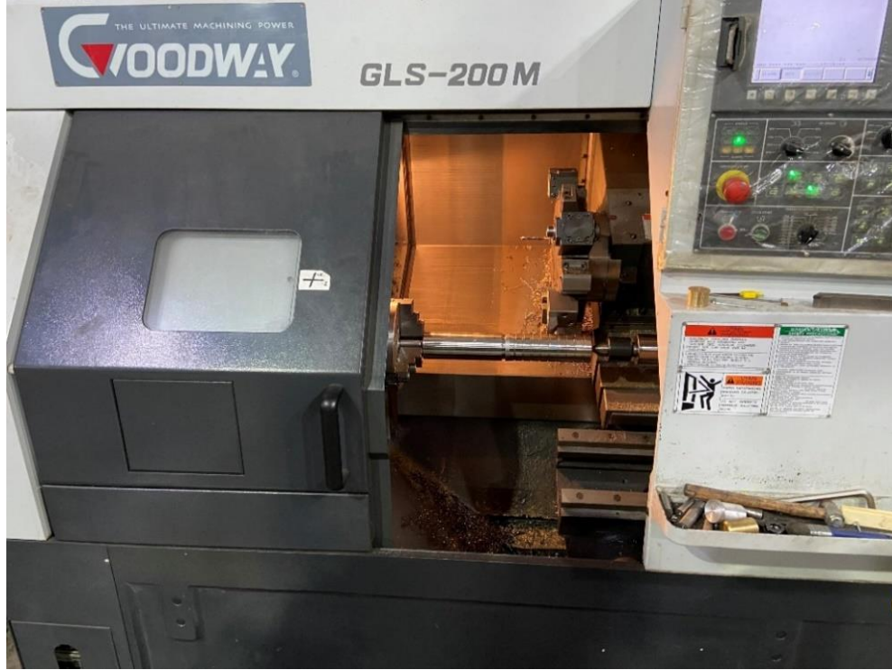
Figure 4.1 CNC Lathe Machine GLS-200 M
