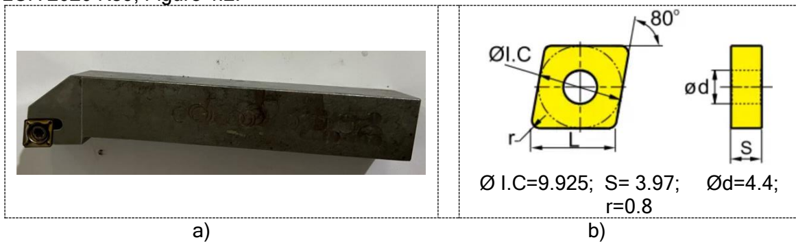
Figure 4. 2. a) Toolholder SCLCR 2020 K89 - Techno Takim, b) Cutting insert CCMT 09T308N
